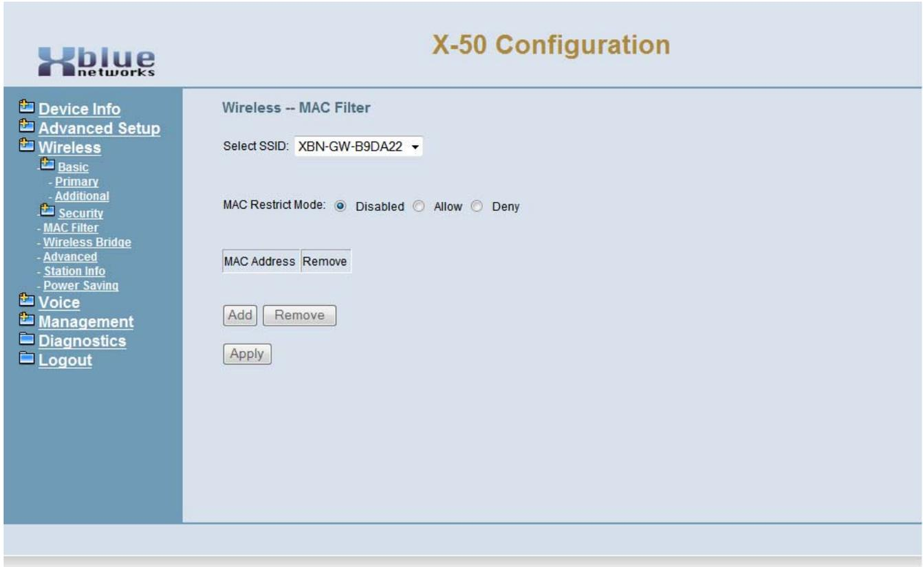
Select “Wireless MAC Filtering”, and then select “Add” to add a MAC address or “Remove” to remove servers from the current list.
