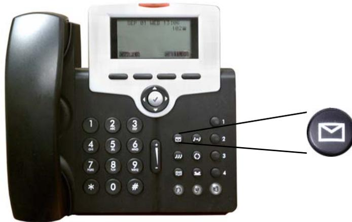
When a new message arrives, the light above the display will begin flashing and the display will show an envelope with the new message count.
