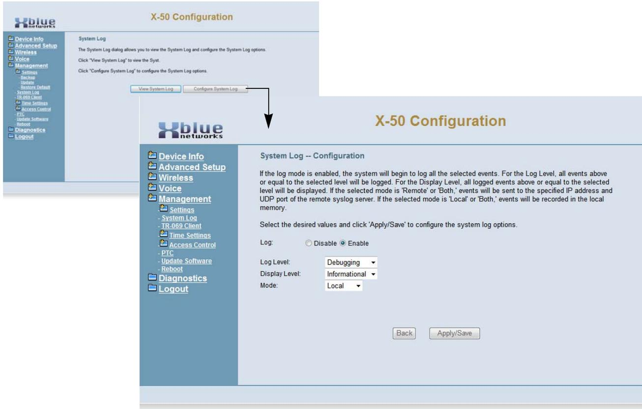
Select "Configure System" log to select the level of logging required.
