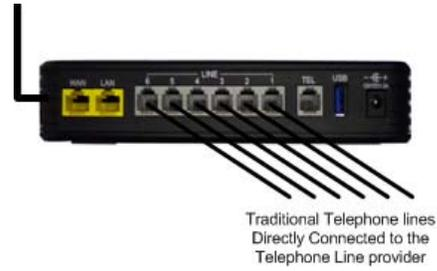
Unlike analog trunks, SIP trunks do not physically connect to the **X-50** VoIP Telephone System. Each SIP trunk is assigned a special authentication ID and Password, that systemically connects them from the SIP Telephone Line provider to the **X-50** VoIP Telephone System using the broadband (Internet) Connection. Once programmed, the **X-50** system and the SIP trunks remain "connected" and are accessed just like an analog trunk.
